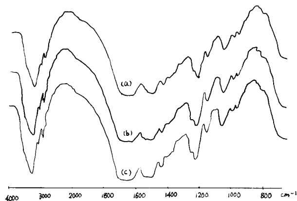
Figure 2 Transmission IR spectra for (a) control silk, (b) air plasma-treated silk, (c) AAm plasma-grafted silk by method (A).
